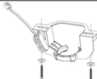
**NOTE:** The mounting screws included in the package are intended for use in wooden structures. For constructions from other material, e.g. concrete structures, the appropriate type of screw should be used.
