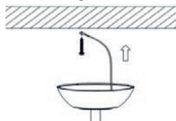
6. Place the remote control receiver between the mounting base and the ball joint as shown below:
