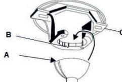
5. For maximum safety, attach the supplied safety cable, ideally to a point independent of the fixing point, or for example to a hook screw on a concrete ceiling.
