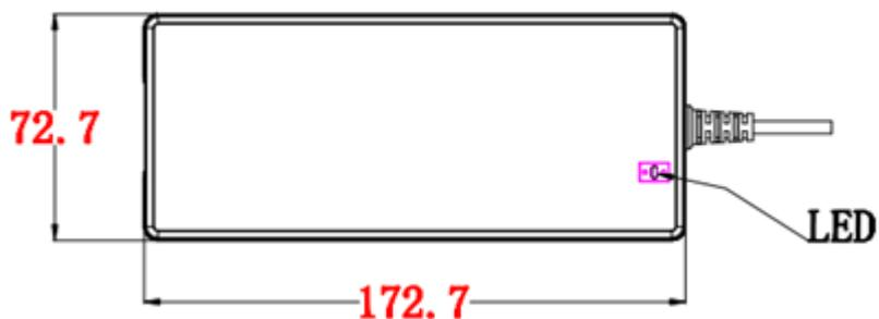
The model AP-PN120-24 charger by natural air. The input voltage range is 100-240Vac, the single-channel voltage is up to 29.2V, and the maximum current is 4A. The power supply has reverse polarity protection. The entire power supply is designed in strict accordance with safety regulations.
