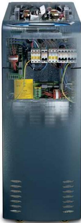
SENTRY MULTISTANDARD series includes 10-15-20kVA single/singlephase, three/single-phase and 10-15-20-30-40-60-80 kVA three-phase models, and uses on-line double conversion technology (VFI). The load is powered continuously by the inverter with a filtered, stabilised and regulated sinewave supply. The input and output filters considerably increase the immunity of the load to mains disturbances and surges, even on bypass.
