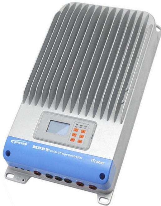
iTracer is an industrial grade product with advanced Maximum Power Point Tracking (MPPT) algorithm. It can deliver the maximum available power for charging batteries and charge a lower nominal voltage battery from a higher nominal voltage array. And can be applied in the off-grid PV systems up to 3KW. The die-cast aluminum design ensures excellent heat dispersion.
